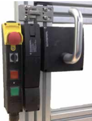
Picture 2: machine controls with emergency stop, mounted at a safety guard access door.
